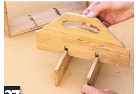
27 Handle and dividers are slotted together. Mark out halving joints and carefully cut away waste
